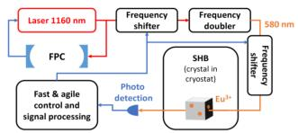
At the SYRTE laboratory, an experimental setup using an  $Eu^{3+}$ :Y<sub>2</sub>SiO<sub>5</sub> crystal has been constructed and the first demonstration of laser stabilization yields a relative frequency stability at a few 10<sup>-15</sup> around 1 s. On-going collaborations with Institut Néel have led to the fabrication of a micro-mechanical resonator made of the same kind of crystal.
