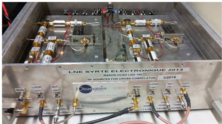
Low noise frequency chains for clock signals
