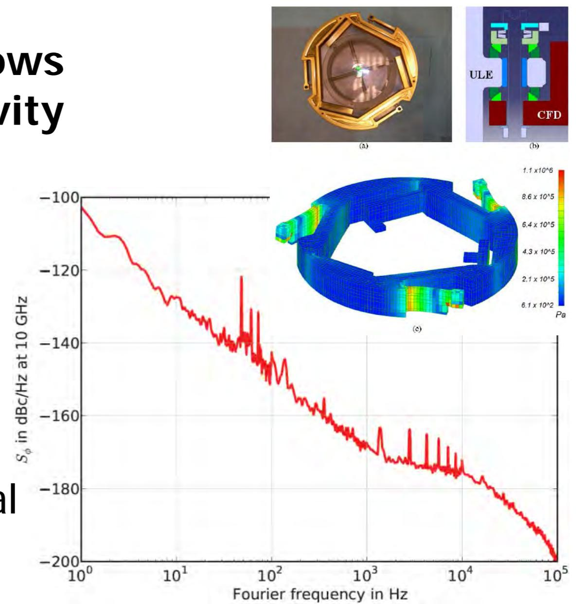
$\phi$ -noise PSD @ 10 GHz carrier from USL at 200THz (ideal division)
