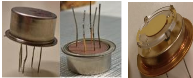
Quartz plate mounted resonator
