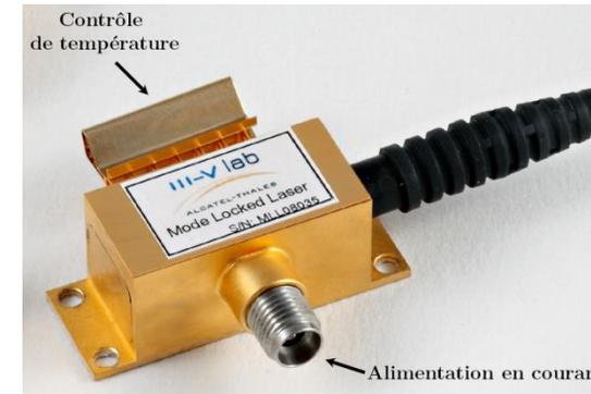
Q-dash Fabry-Perot Mode Locked Laser Diode
