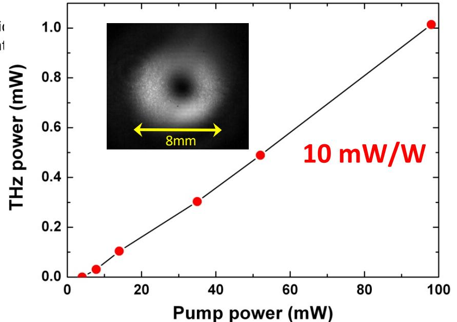
Maximum theoretical efficiency: 18.5 mW/W
