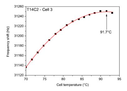
Cs clock frequency versus the temperature in a Cs-He microcell. An inversion temperature is obtained in this case at 91.7°C.
