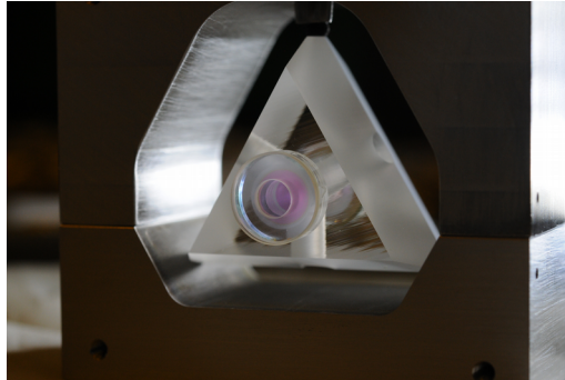
Compact ULE cavity in its stainless steel spacer.
