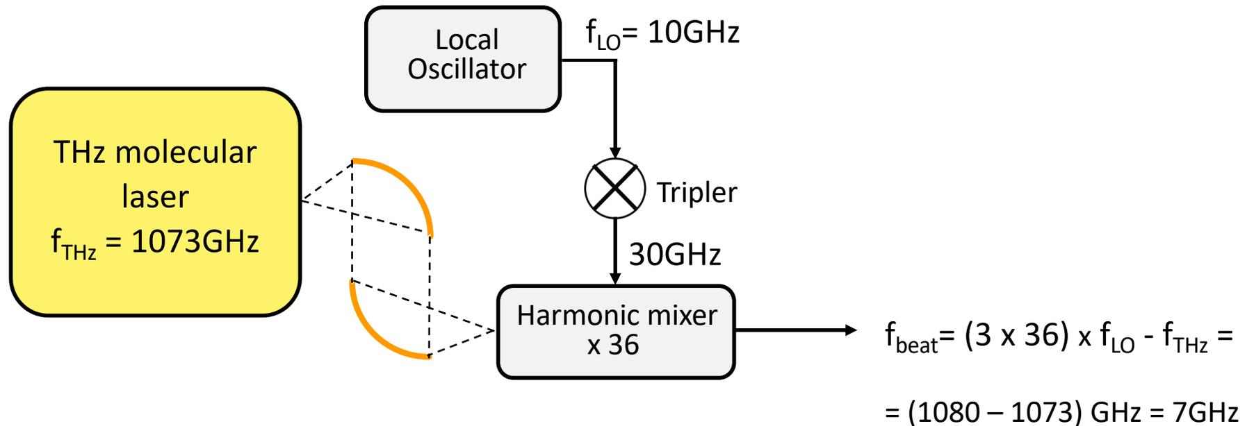
$$|\delta f_{\text{beat}}|_{\text{rms}} = 108 \times |\delta f_{LO}|_{\text{rms}} + |\delta f_{\text{THz}}|_{\text{rms}}$$
